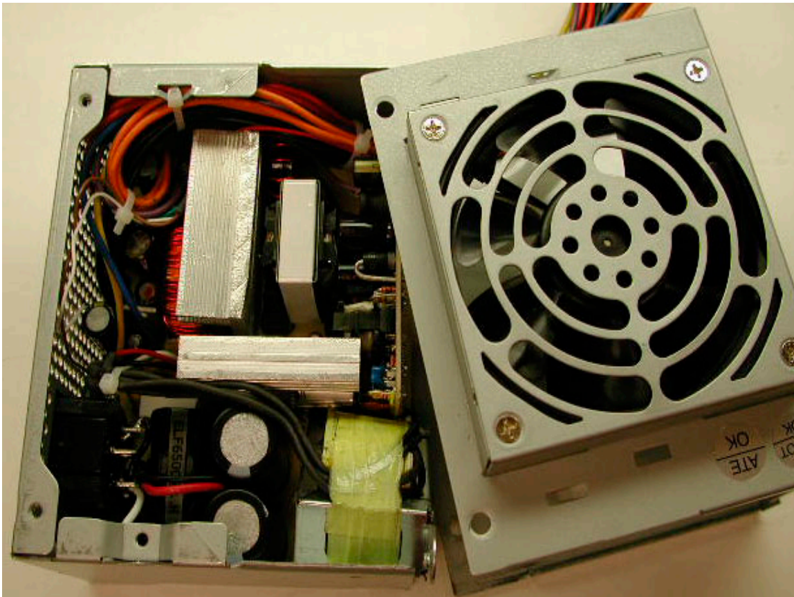
Figure 1 – Photograph of the populated circuit boards of the EP-31 prototype.
